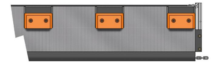
Beach Bouncer - Type III is a seaweed control barrier that consists of a heavy duty coated mesh barrier supported by molded hard floats. It features a stainless steel load carrying cable and ballast at the bottom of the skirt. This construction allows for ready servicing of the field with easy replacement of the floats or base fabric.
